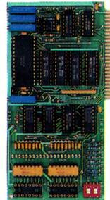
**12 bit, 16 channel, programmable gain A/D** Monitor flow, temperature, wind speed and direction, humidity, light intensity, pressure, RPM, soil moisture and many other conditions. Our complete 12 bit A/D converter has 16 single-ended full scale ranges from  $\pm 10$  volts to  $\pm 25$  MV. Other features include very fast (.025 ms) conversion time and a user connector with +12 and -12 volts for powering your sensors. **\$279**
